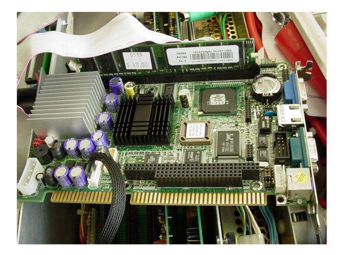
With this new SBC I was able to eliminate the old VGA to TFT card configuring the new TFT connection directly from the SBC.
