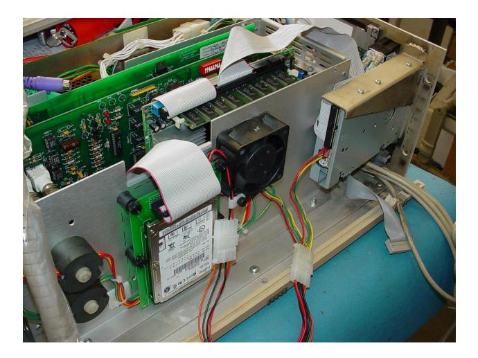
Because some of the old full sized IDE Hard Drives were getting broken heads when the operators would tip the testers over, I had a mounting plate adaptor built for the much more durable mobile laptop drive. Than I would install the whole assembly on shock mounts.
