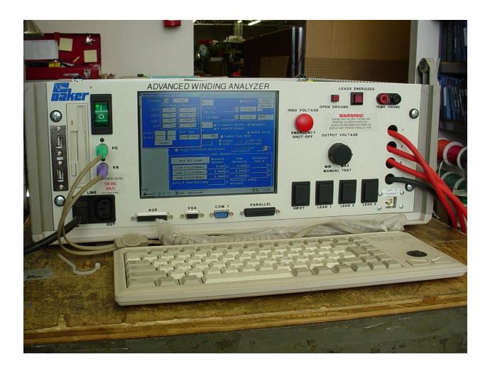
This was an old AWA-II that I upgraded back in 2004 It originally shipped with win N/T OS and I installed a new faster motherboard, windows 2000 with new USB & CAT-5 ports.
