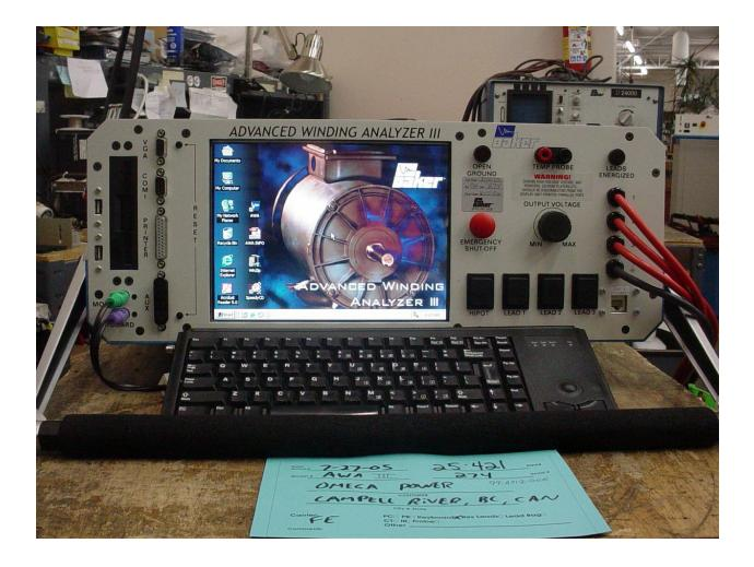
This was an old AWA-III That I upgraded back in 2005. With a new faster SBC Motherboard and a new Hard drive with an updated Operating System
