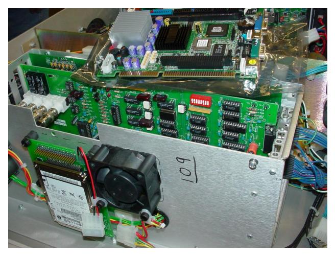
With this new SBC I was able to eliminate the old VGA to TFT card configuring the new TFT connection directly from the SBC.
