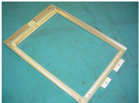
I designed a new LCD Bezel to incorporate a touch screen in front of the LCD. Back in 2005 a touch screen was cutting edge for a tester.
