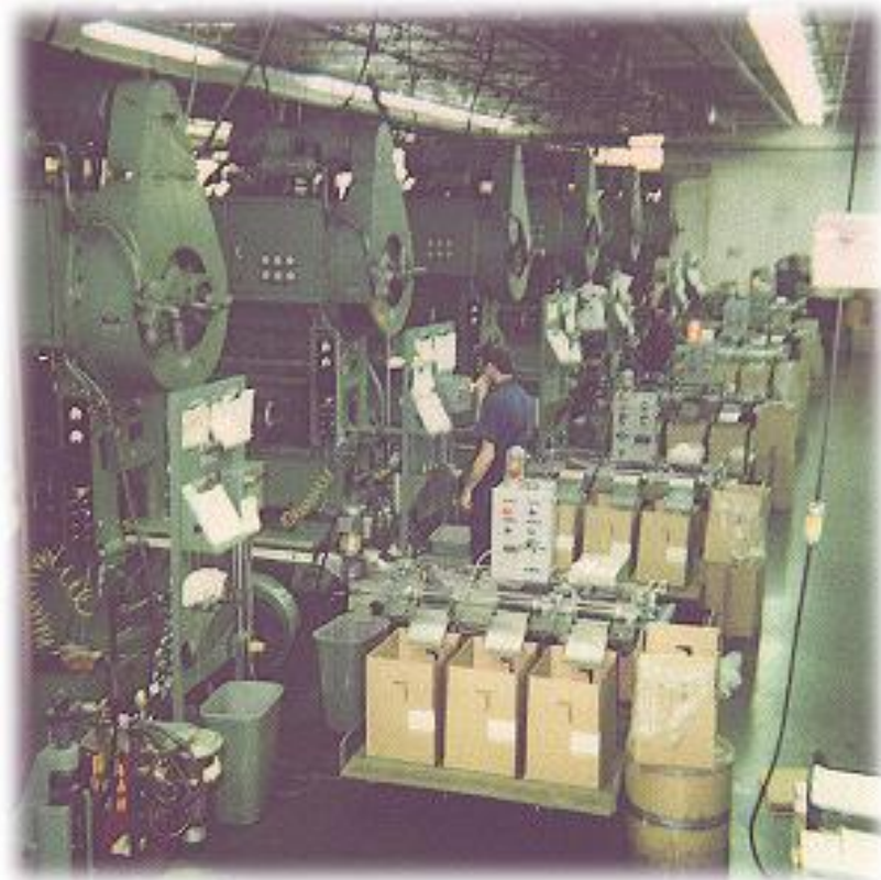
This shows the box conveyors that I designed and fabricated, which added 68% increase in production.
