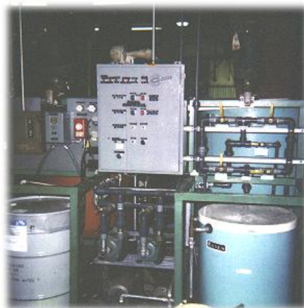
This is the white lube control system, for lubricating the steel with metered precision as it fed into the press at 350 spm. I designed, built and programmed this system.
