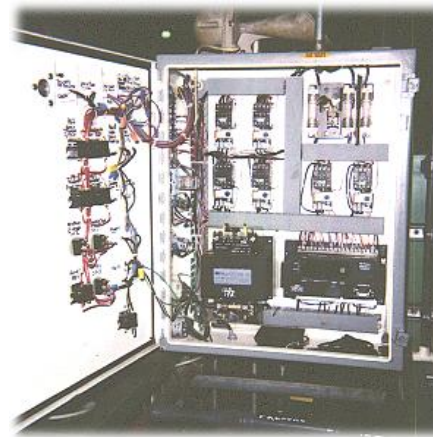
This is the white lube control system, for lubricating the steel with metered precision as it fed into the press at 350 spm. I designed, built and programmed this system.
