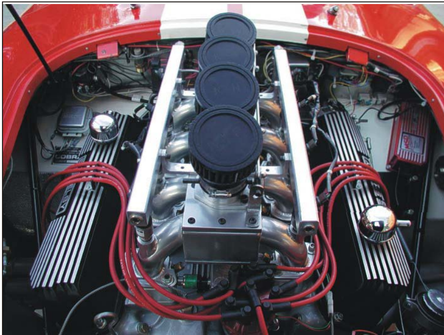
Figure 3-6 Hydrogen Internal Combustion Engine
